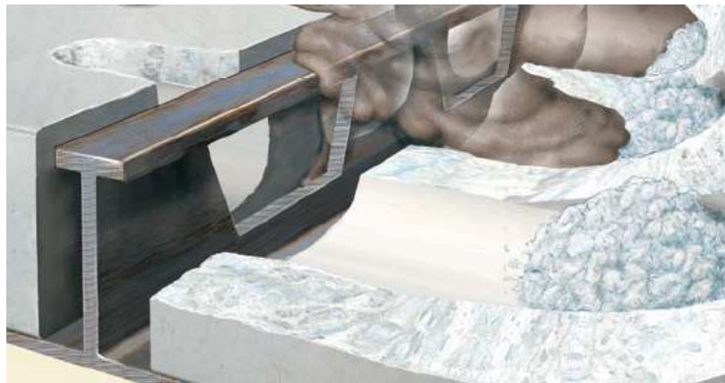
Figure 2.2 – Typical Girder-Slab Floor System (Girder-Slab Technologies, 2008)
