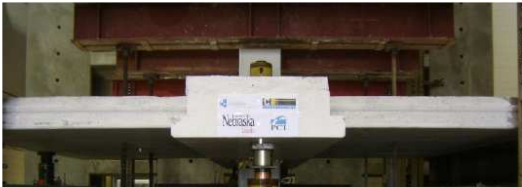
Figure 2.4 – Shallow Hollow-Core Floor System (Tadros and Morcous, 2011)
